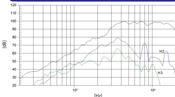
Note: On axis frequency response measured in anechoic chamber, 1W @ 1m
